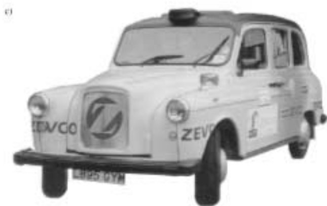
Figure 24. Fuel cells used in vehicular systems: a) NECAR 4 (Daimler–Chrysler); b) Demio FCEV (Mazda); c) an alkaline fuel cell vehicle (the ZEVCO London Cab).
