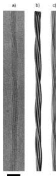
Figure 3. a) Cryo-TEM picture of one C8O3 J-aggregate that consists of five single strands. b) A simple model, that consists of a bundle of tubules that are packed on a trigonal lattice and twisted around each other. c) The calculated image of the J-aggregate, derived from the model in (b). The scale bar corresponds to 50 nm.
